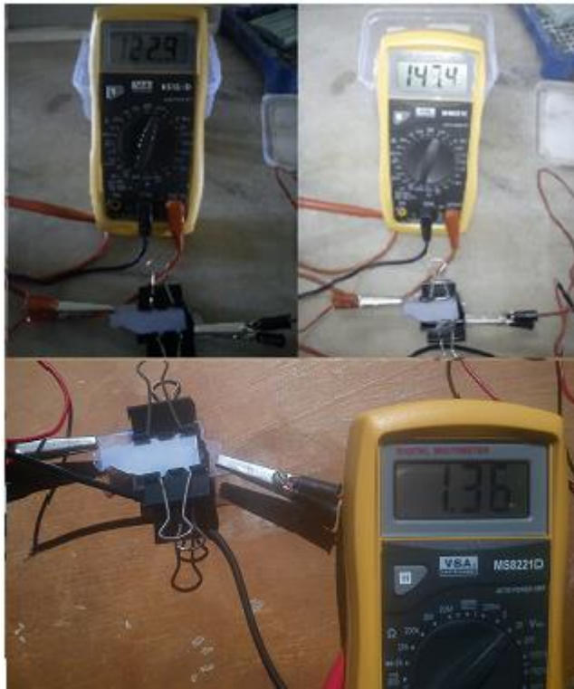
Figure. 7 Testing of DSSC a) In normal light b) In torch light c) In bright sun light
